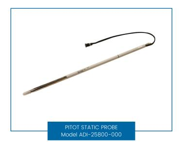
The Pitot Static Probe (PSP) was tested to provide dynamic and static pressures for speed and altitude respectively up to 125kts and 25,000fts and under the most severe icing conditions (FAR-25 C).
