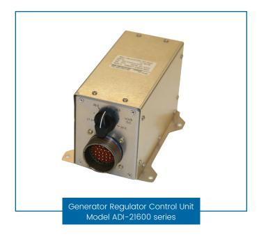
The Generator Regulator Control Unit (GRCU) provides generator field excitation and regulation functions for the main 28 VDC bus system of an aircraft. The GRCU is designed to operate in harsh vibration as well as harsh electromagnetic environments such as HIRF and severe indirect lightning. The GRCU functions include twin-engine starter-generator cross-start, voltage regulation, redundant overvoltage protection, and automatic bus switching.
